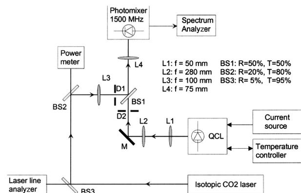
Fig. 1. Schematic of the optical setup for the beating experiment: BS1–BS3, beam splitters; L1–L3, lenses; D1, D2, beam waists; M, mirror.
