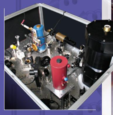
laboratory the very first LHR with a wide spectral coverage allowing the monitoring of several gases rather than a few, thus, greatly increasing the remote sensing capabilities of the instrument. With further funding, the project team will shortly undertake atmospheric demonstration of the multi-species monitoring capabilities.
