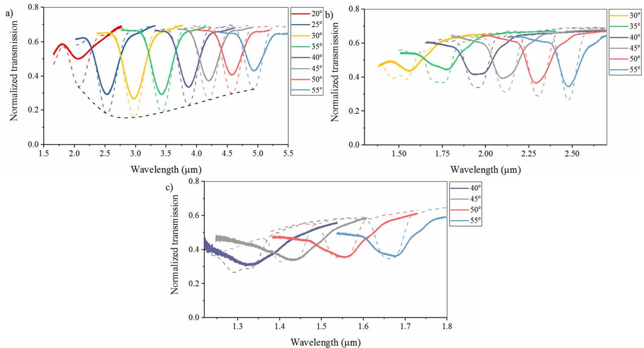
Figure 3. Measured (solid) and modeled (dashed) data for first (a), second (b) and third (c) order diffraction of a grating designed for peak first order diffraction at  $3 \mu\text{m}$ .
