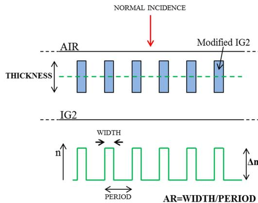
Figure 2. Definition of model parameters. Green dashed cross-section in upper image has the refractive index profile shown in green in the lower part of the figure.
