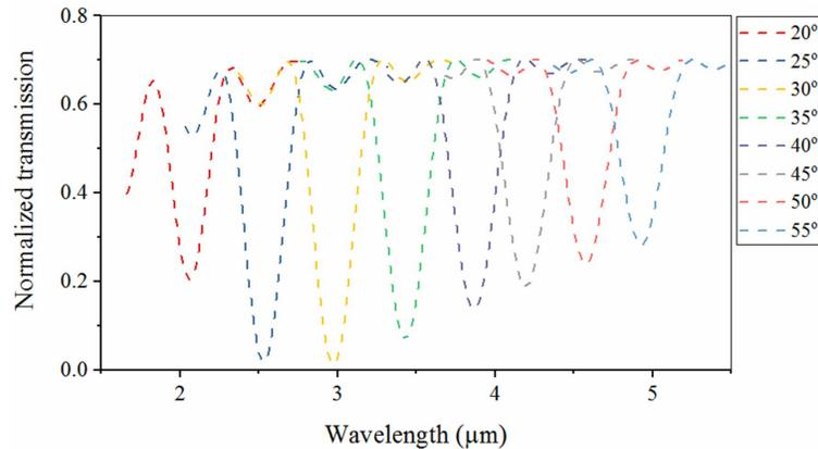
Figure 4. Modeled spectra for a single angle of incidence (collimated beam), showing close to 70% first order diffraction efficiency at the peak diffraction wavelength.
