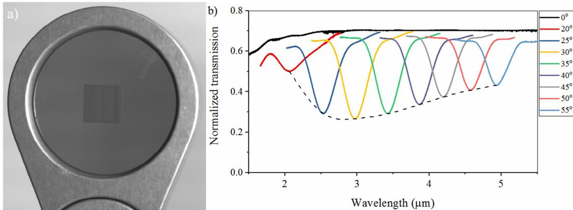
Figure 1. (a) Photograph of a fabricated IG2 grating structure, obtained under near-infrared illumination. (b) Zeroth order transmission spectra of IG2 transmission grating designed for peak diffraction wavelength at 3  $\mu\text{m}$ . Plots are truncated to show only the first diffraction order dips.
