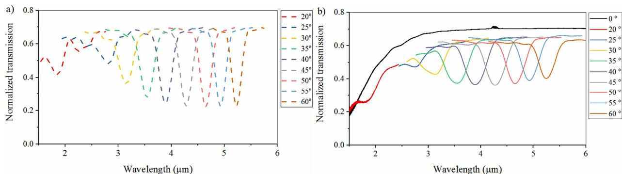
Figure 5. Modeled (a) and measured (b) data for a grating designed for peak first order diffraction at  $4.3 \mu\text{m}$ .
